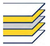
Release Liner Adhesive Carrier Adhesive Release Liner
